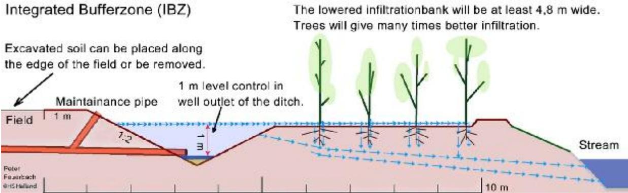
**Figure 2** – A cross section of a typical Integrated Buffer Zone.
